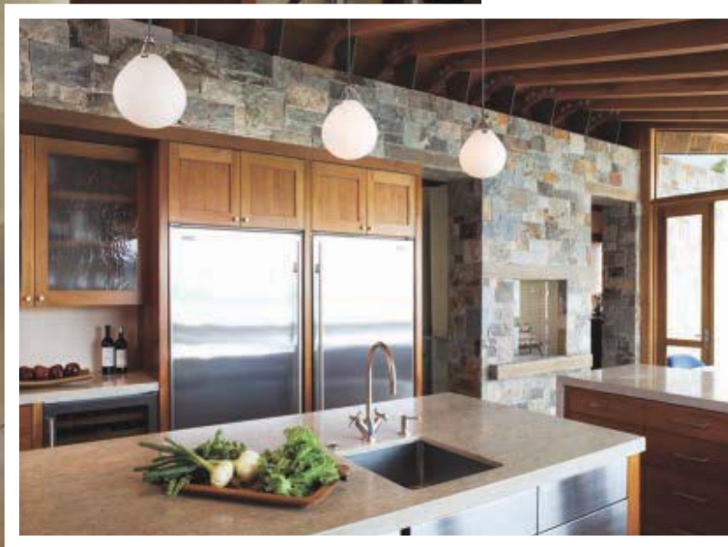
Architect Ron Sutton (above) with his client, interior designer Andra Martens, chose a central wall of Montana ledge stone that not only provides thermal mass but adds dramatic texture to every room, including the kitchen where it abuts the wood rafters.
